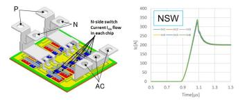
Figure 4: Simulation result of current sharing at turn-on event in LV100 package concept.
