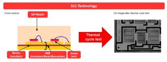
Figure 5: SLC-Technology and thermal cycle test result
