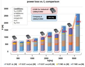
Figure 6: Power loss comparison of 7th gen. IGBT chip in LV100 1200A/1700V module vs. Company A 1400A/1700V conventional module.
