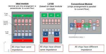
Figure 3: Comparison of power module layout concepts
