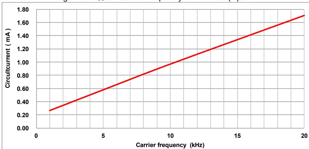
Fig. 4-2-3.  $I_{DB}$  vs. Carrier frequency for PSS15M(N)C1FT
