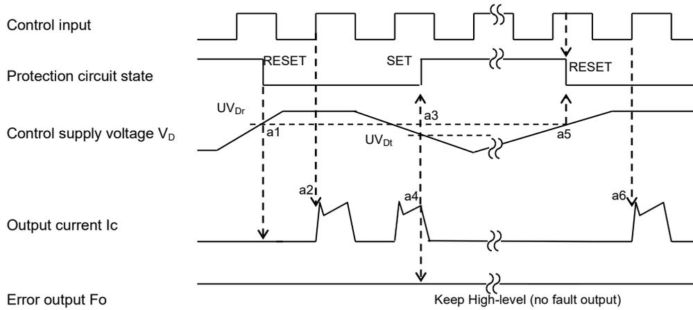
Fig.2-2-6 Timing Chart of brake circuit UV protection
