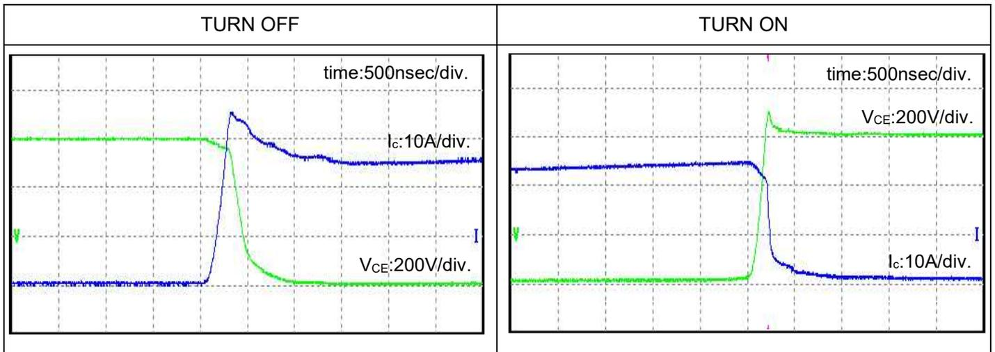
Fig. 2-1-5 Typical switching waveform for PSS25MC1FT (25A/1200V) inverter part
