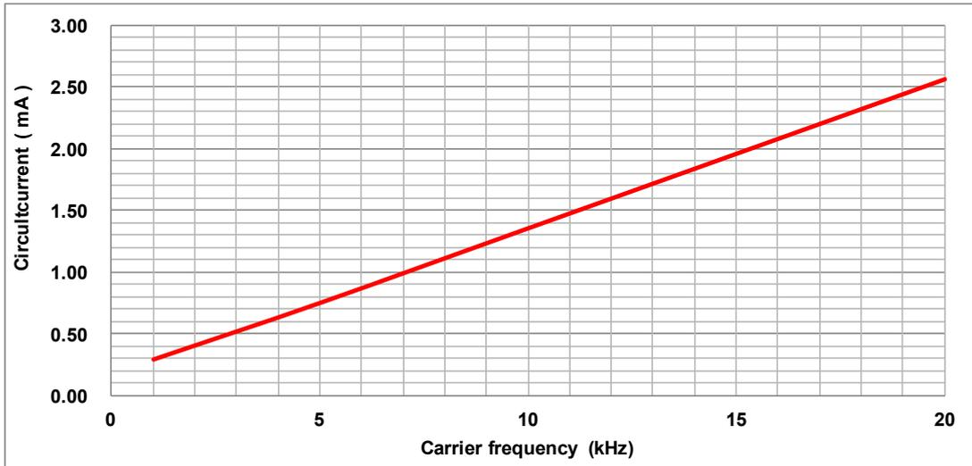
Fig. 4-2-4. I<sub>DB</sub> vs. Carrier frequency for PSS25M(N)C1FT
