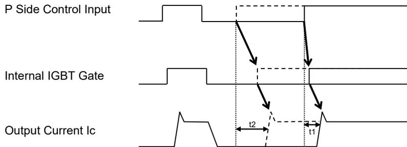
Real line...off pulse width > PWIN(off); turn on time t1
