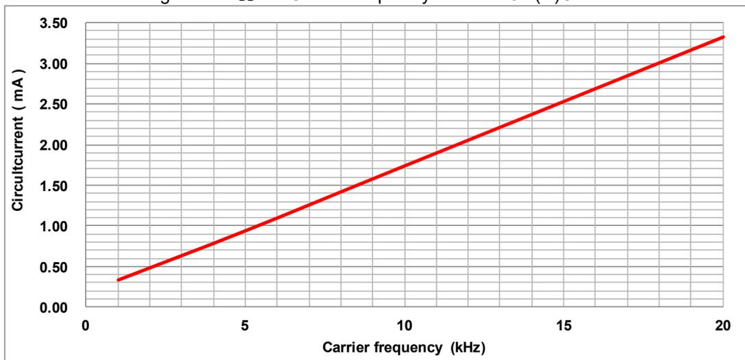
Fig. 4-2-5. I<sub>DB</sub> vs. Carrier frequency for PSS35M(N)C1FT
