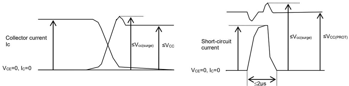
Fig.3-1-13 SOA at switching mode and short-circuit mode
