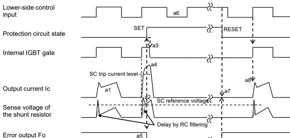
Fig.2-2-3 SC protection timing chart
