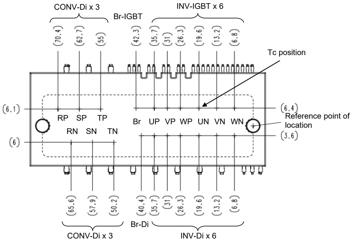
Fig. 2-1-1 Power chips layout (Unit : mm)
