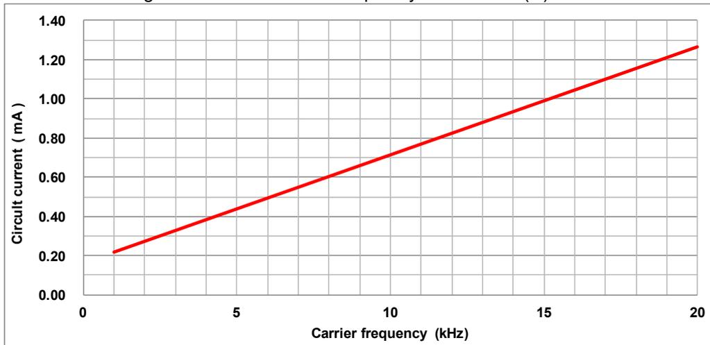
Fig. 4-2-2.  $I_{DB}$  vs. Carrier frequency for PSS10M(N)C1FT
