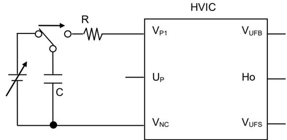
Fig.3-3-4 Surge test circuit example (V<sub>P1</sub> terminal)
