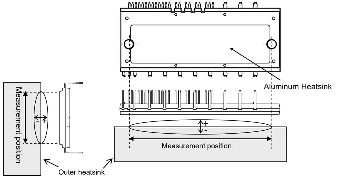
Fig.2-4-2 Measurement positions of heat radiation part flatness
