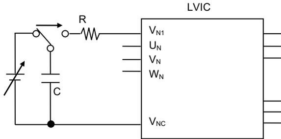
Fig.3-3-3 Surge test circuit example (V<sub>N1</sub> terminal)
