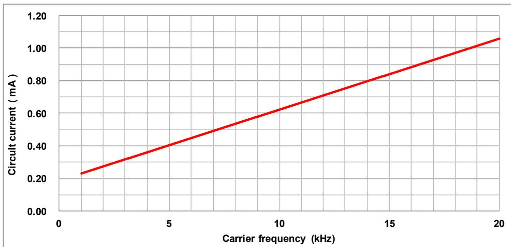
Fig. 4-2-1.  $I_{DB}$  vs. Carrier frequency for PSS05M(N)C1FT
