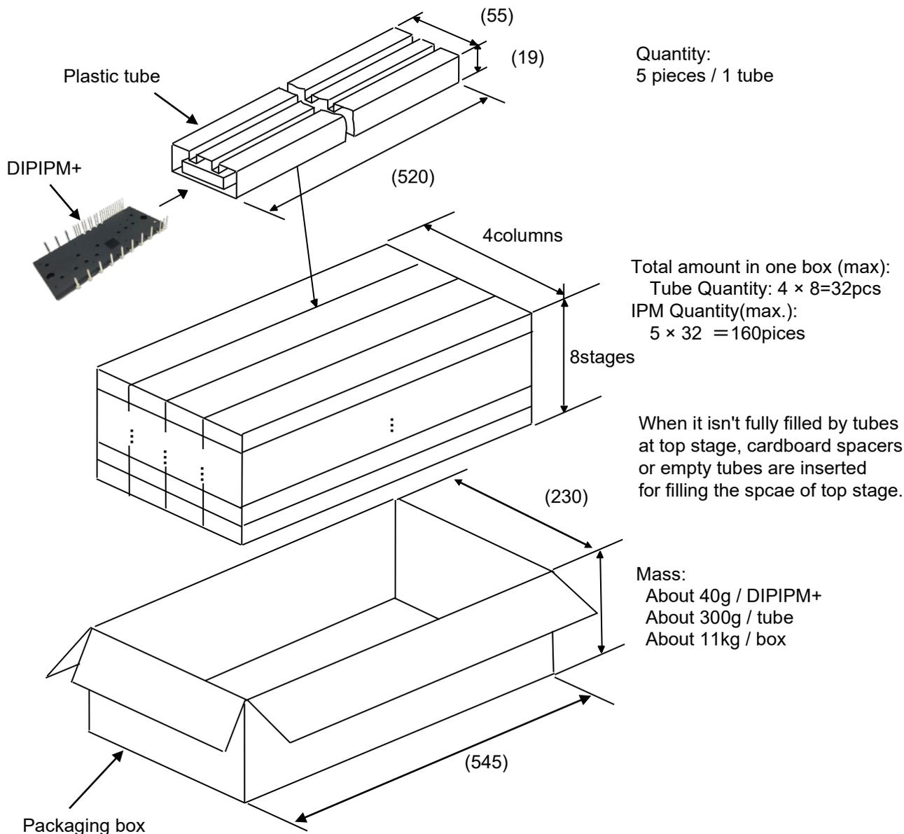
Spacers are put on the top and bottom of the box. If there is some space on top of the box, additional buffer materials are also inserted.
