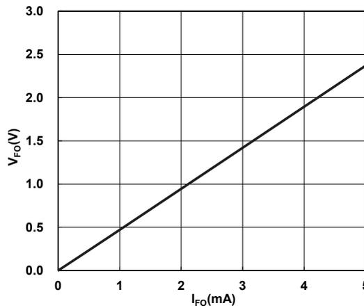
Fig.3-1-8 Fo terminal typical V-I characteristics ( $V_D=15V, T_j=25^{\circ}C$ )
