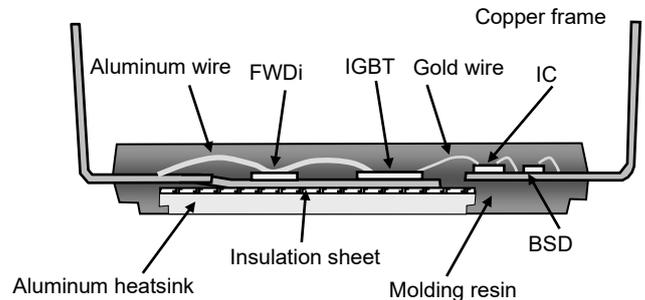
Fig. 1-2 Cross-sectional structure
