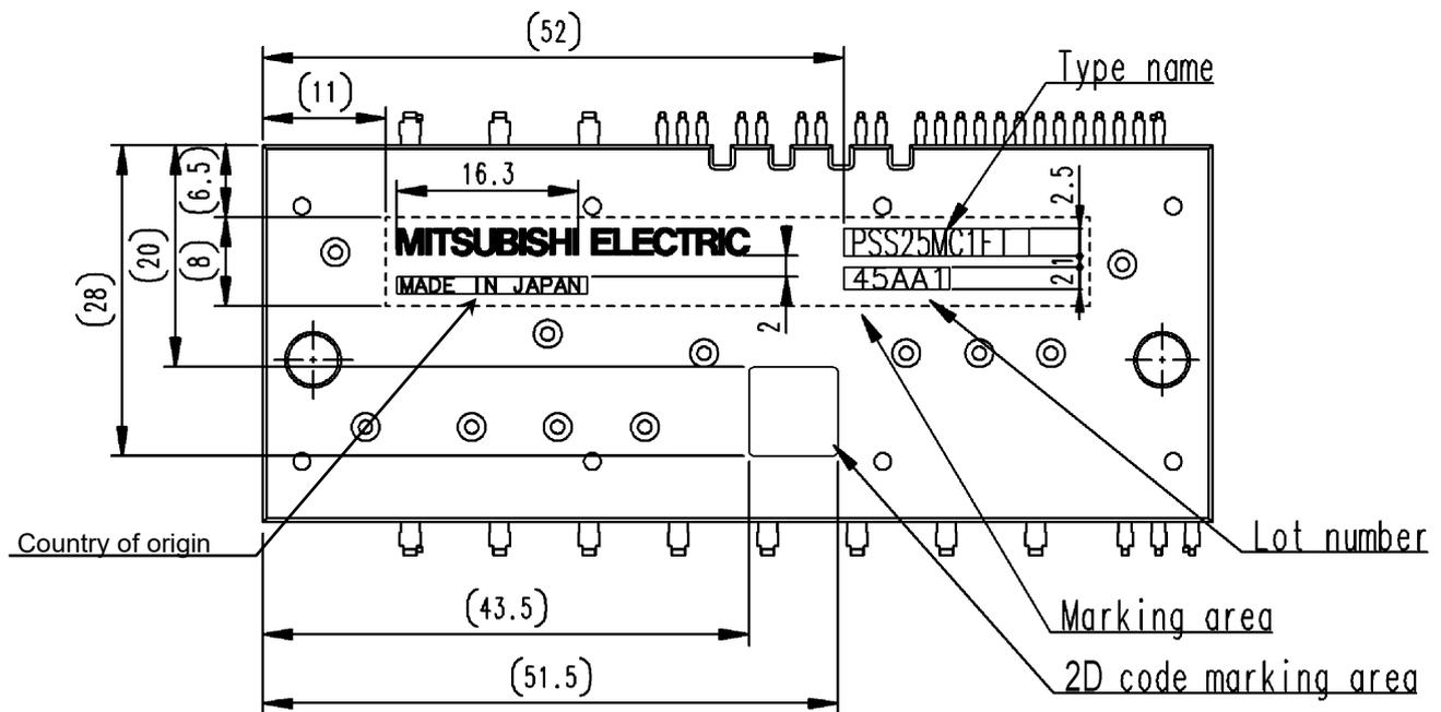
Fig.2-3-2 Laser marking view PSSxxxC1Fx (Dimension in mm)
