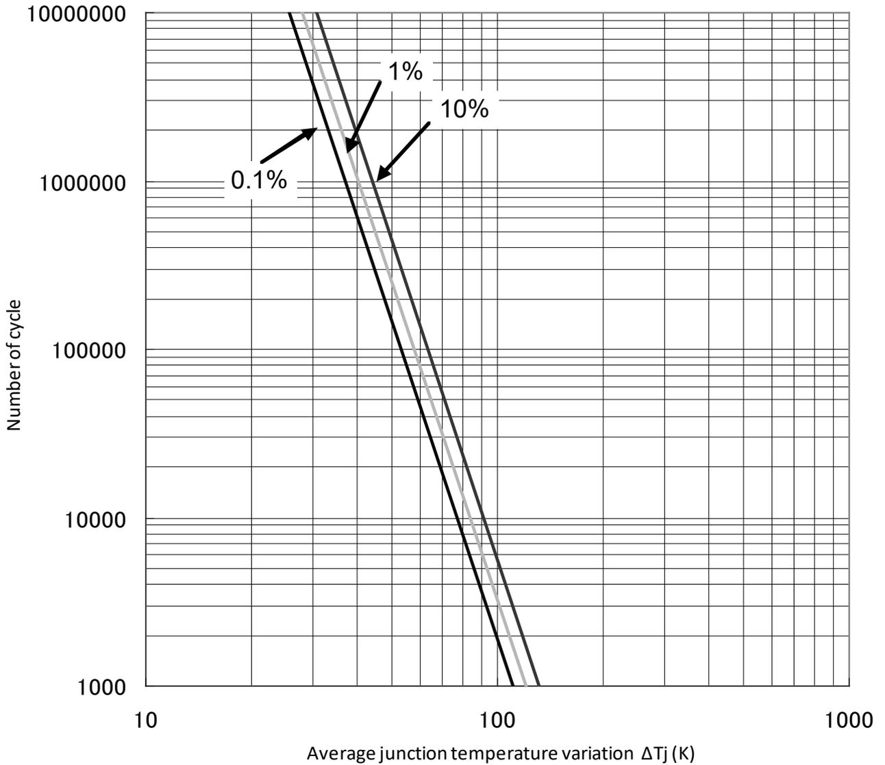
Fig.3-1-20 Power cycle curve
