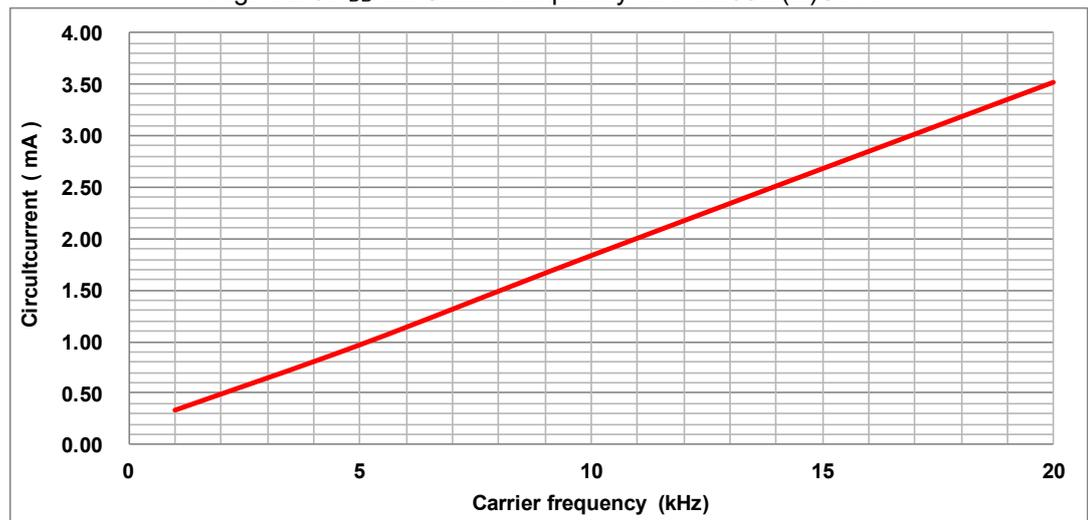
Fig. 4-2-6. I<sub>DB</sub> vs. Carrier frequency for PSS50M(N)C1F6
