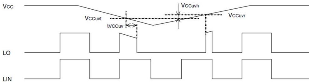
If V<sub>CC</sub> supply voltage drops below UV trip voltage (V<sub>CCuvt</sub>) for V<sub>CC</sub> supply UV filter time, HO output signal is shut down. And then, if V<sub>CC</sub> supply voltage rises over UV reset voltage, HO will return to the usual operation mode.
