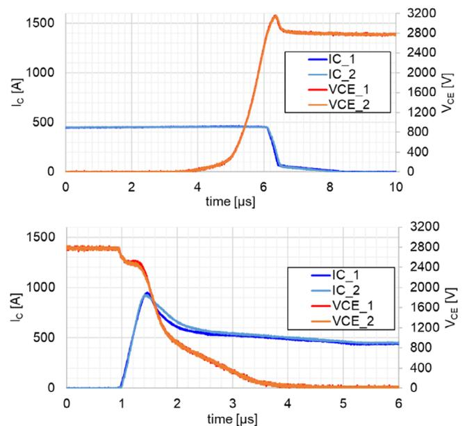
Figure 7: Current sharing of two parallel-connected CM450DE-90X (Conditions:  $V_{CC}=2800\text{ V}$ ,  $I_{C,total}=900\text{ A}$ ,  $V_{GE}=\pm 15\text{ V}$ ,  $T_j=25^\circ\text{C}$ , N-side)
