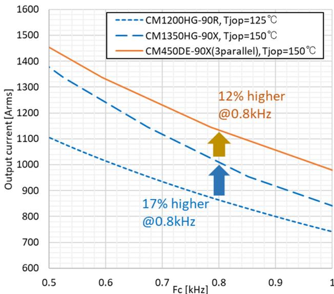
Figure 5: Relationship between output current and carrier frequency for R series HVIGBT, X series HVIGBT and 4.5kV HV100 (Condition: Sinusoidal,  $V_{CC}=2800\text{ V}$ ,  $P_f=+0.85$ ,  $M=1$ ,  $T_s=80^\circ\text{C}$ ,  $T_j = T_{jop}$ )
