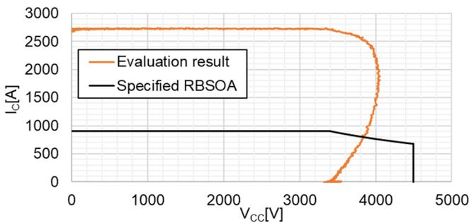
Figure 9: Specified RBSOA and evaluation result ( $V_{CC}=3400\text{V}$ ,  $T_J=150^\circ\text{C}$ )
