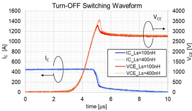
Figure 8: Comparison of switching waveform of 4.5kV HV100 between  $L_S=100\text{nH}$  and  $L_S=400\text{nH}$  (Condition:  $V_{CC}=2800\text{V}$ ,  $I_C=450\text{A}$ ,  $V_{GE}=15\text{V}$ ,  $T_J=150^\circ\text{C}$ )
