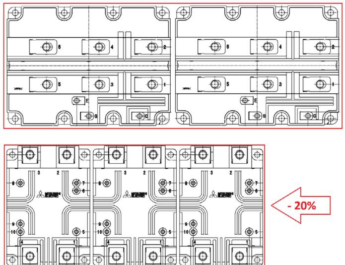
Figure 3: Size comparison for one half bridge with HV100 and conventional packages at same nominal current rating
