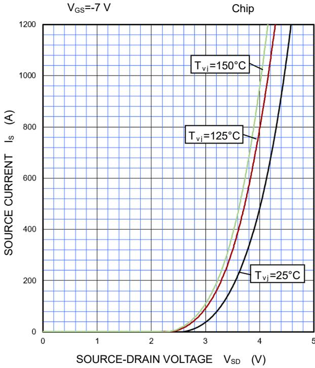
SOURCE-DRAIN ON STATE VOLTAGE
