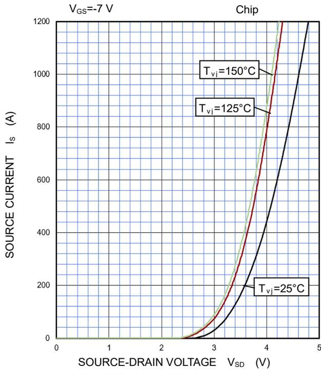
SOURCE-DRAIN ON STATE VOLTAGE
