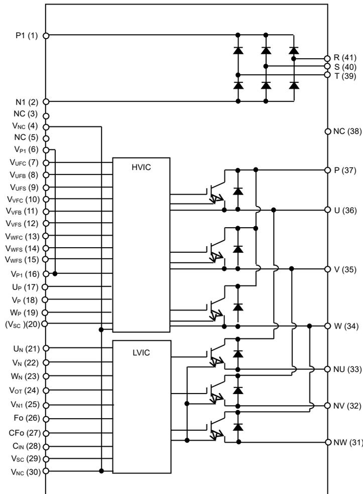
\*It is necessary to short the  $V_{USC}-V_{UFS}$ ,  $V_{VSC}-V_{VFS}$ ,  $V_{WSC}-V_{WFS}$  pins.
