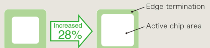
Compared to previous product (CM750HG-130R), the optimized edge termination increases the active chip area by 28 %
